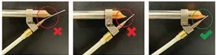
Figure 35: The Nozzle Tip Must Touch the Wire Feed at All Times
