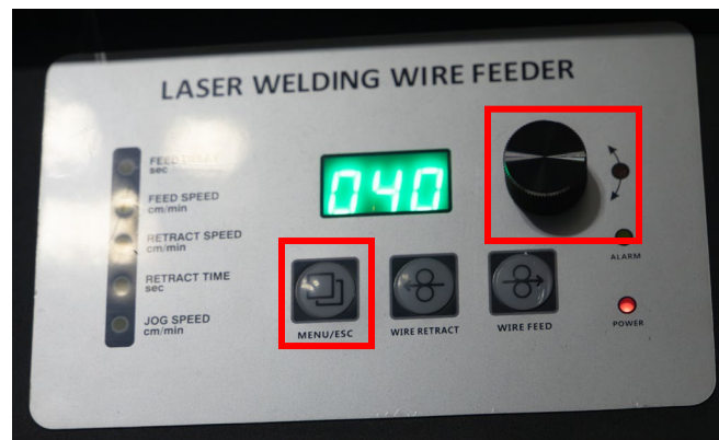
Figure 38: Set the Wire Feed Speed for the Welding Job
