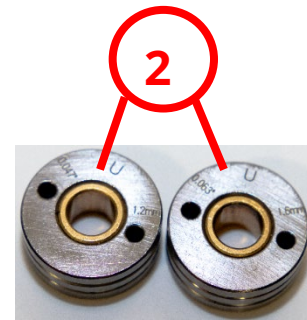
Figure 49: The 0.047"-0.063" U-DRIVE ROLLS
