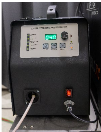
Figure 25: Ensure that the Wire Feeder Attachment is as Straight as Possible
