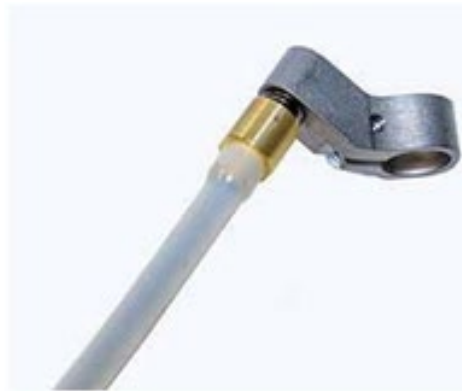
Figure 26: Unscrew the Contact Tip from the Weld Head Adapter
