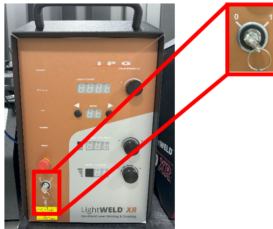
Figure 31: Turn on the LightWELD Unit Using the Switch Key
