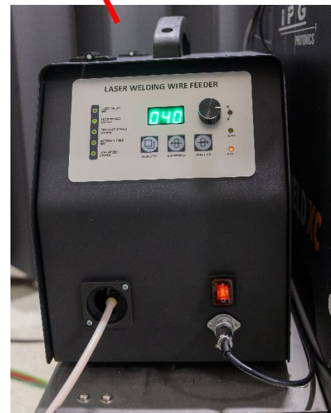
Figure 46: The Wire Feeder Setup Guide and the Wire Feeder Unit
