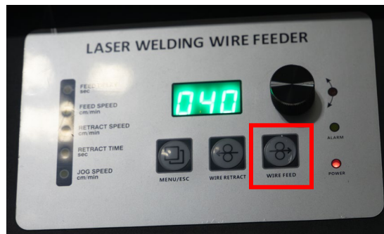
Figure 27: Press the Wire Feed Button
