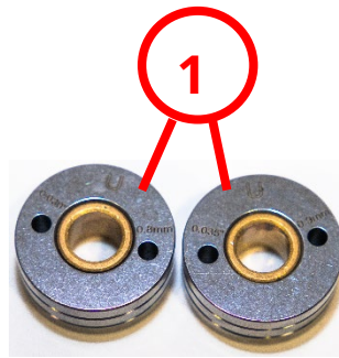
Figure 48: The 0.030" - 0.035" U-DRIVE ROLLS
