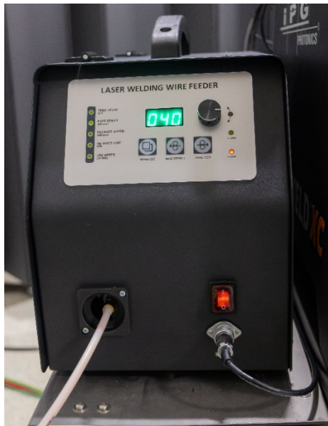
Figure 29: Attach the Synch Cable to the Front of the Wire Feeder
