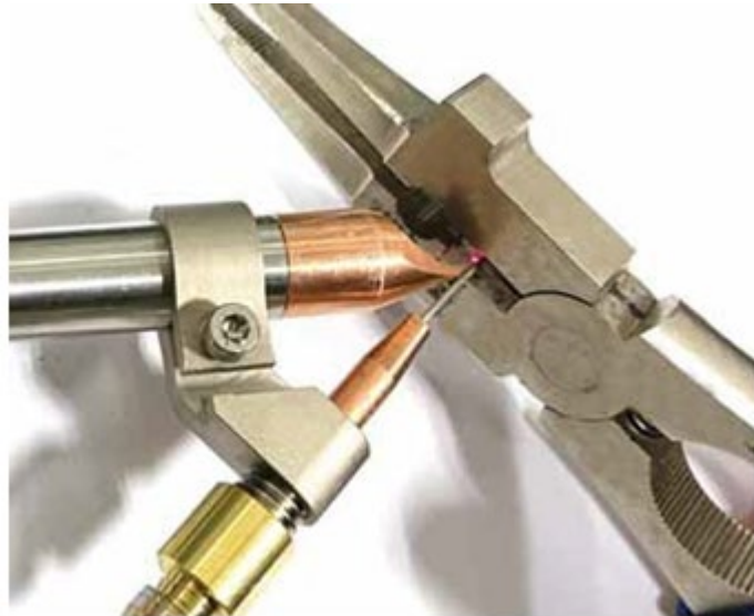
Figure37: Trim the Excess Wire where It Intersects the Guide Beam
