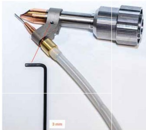
Figure 34: Attach the Weld Head Adapter by Sliding it onto the Tube
