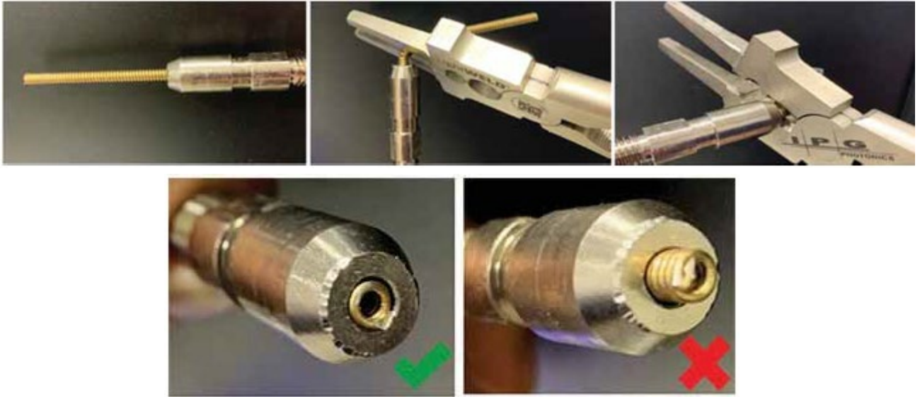
Figure 8: Tighten the Wire Feeder Adapter on the Conduit
